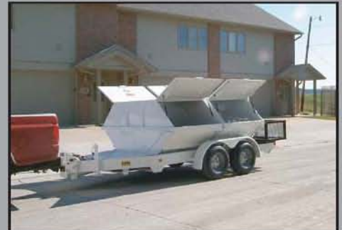
Each of the large side loading containers have dual gas prop assisted top hinge lids for easy loading and unloading.
