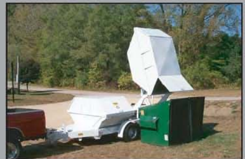
Side Dump containers dump independently.
