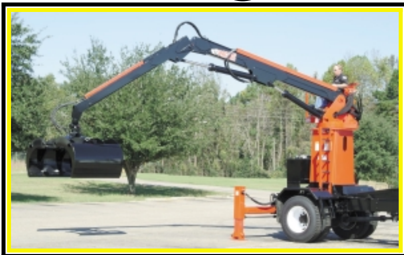
22 ft. Fixed or 25 ft. (3 ft. Extend) Boom Length
