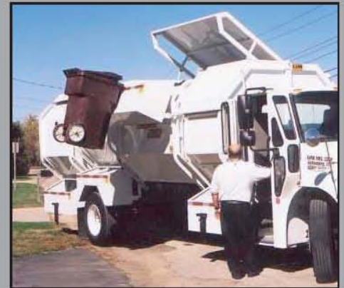
In addition to the troughs, the cart tipper option provides the ability to pick up carts.
