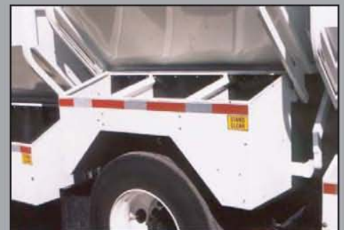
Up to three splits per container and shallow containers are available over axles.
