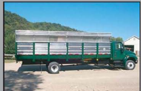
The VERSAHAUL® can be equipped with either a square or v-style plastics cage.
